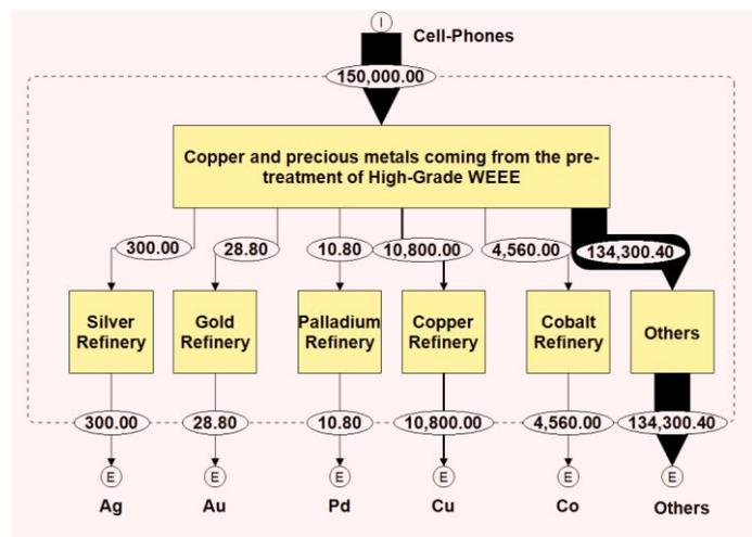
Figure 2. Schematic diagram of global potential recovery of five selected precious metals (Ag, Au, Pd, Cu, Co) from mobile phones (values are reported in Mg/a) [13]
